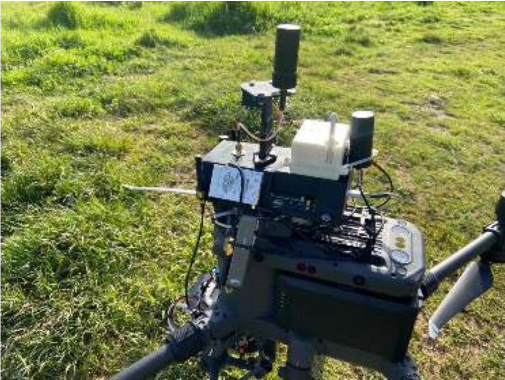
Figure 3-25 – ICARUS Payload installed on DJI M300 RTK UAS
