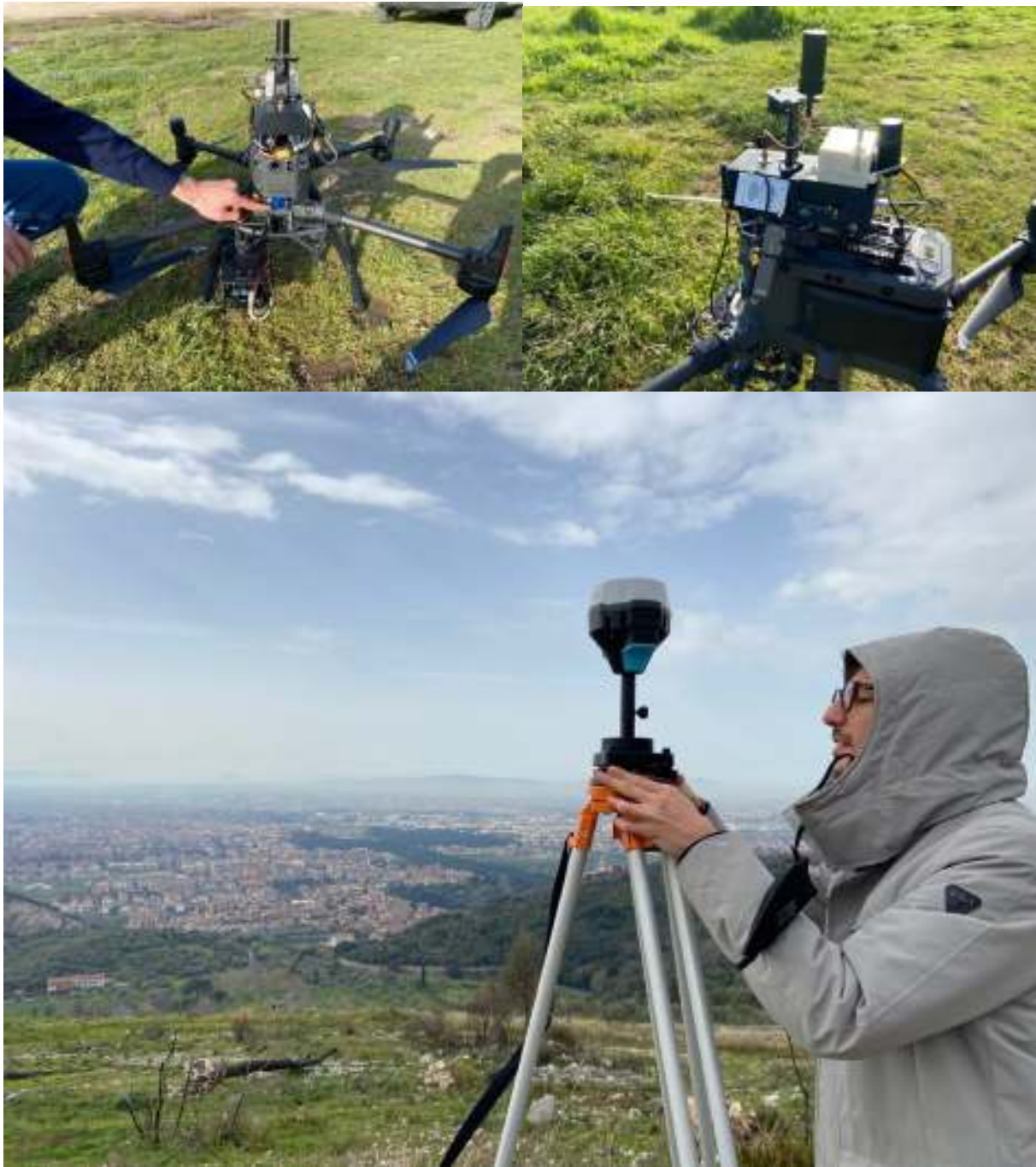
Figure 3-61: Preparation of drones and RTK GNSS station on the test site (300 m AMSL)
