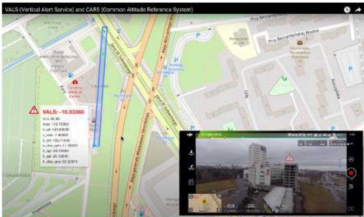
Figure 2-5 – VALS service visualised on Droneradar web application. Caution: The exclamation on DJI mobile app is graphically animated
