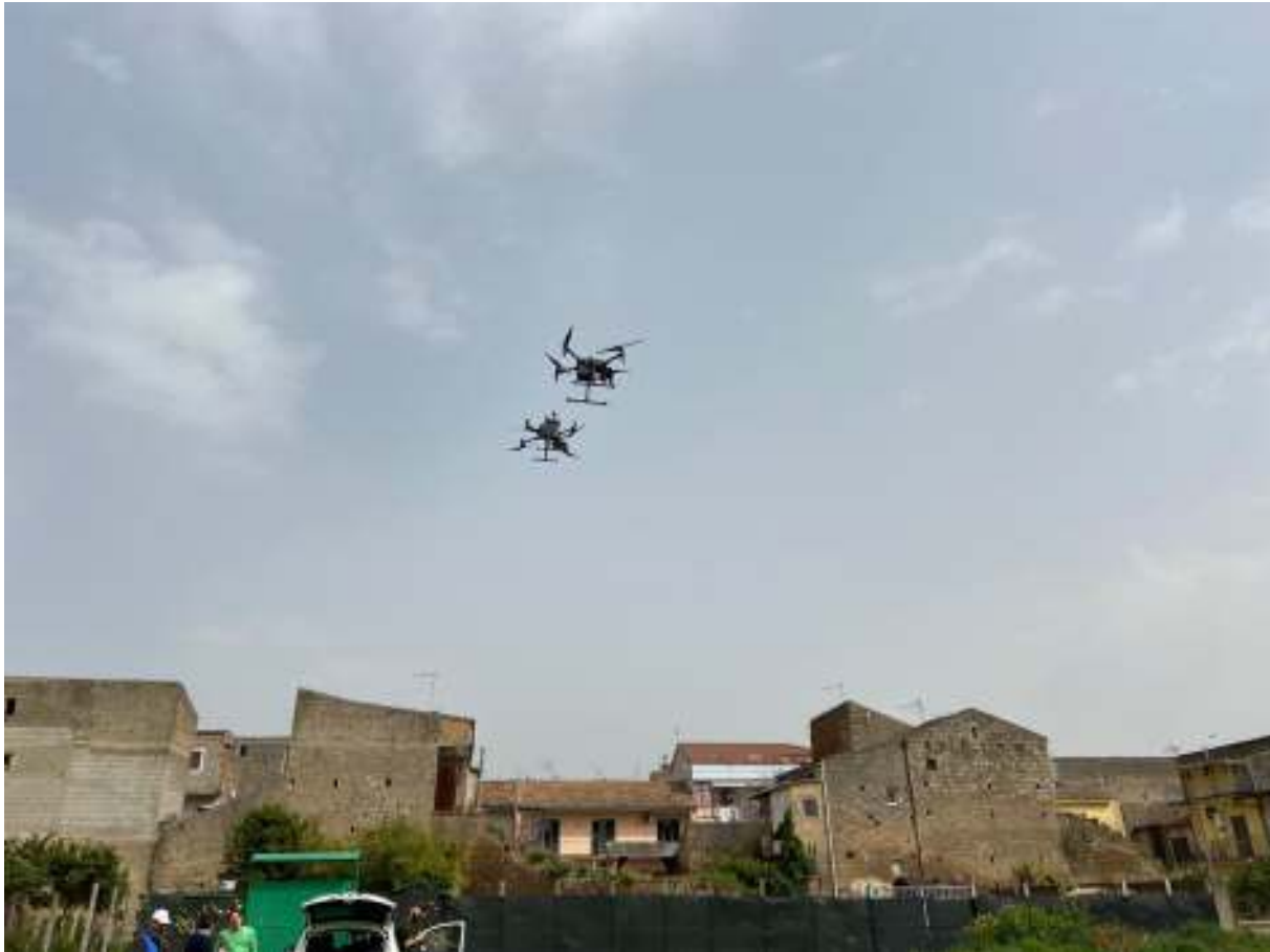
Figure 3-27 – Implementation of test for UAS-UAS vertical accuracy comparison.
