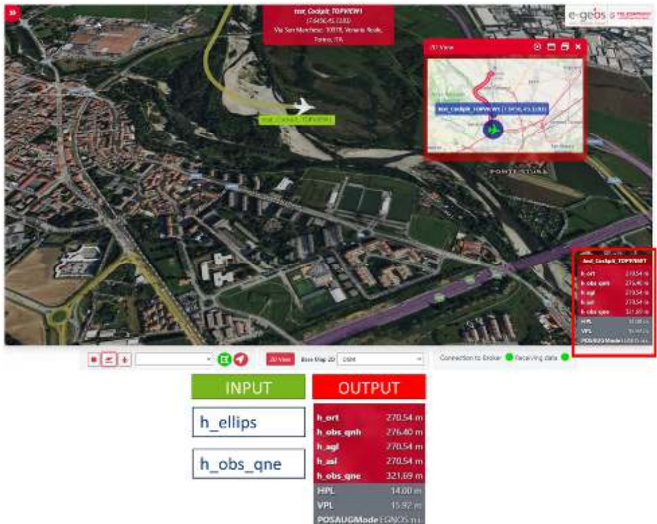
Figure 2-5 –TPZ-E-GEOS SW Platform used for visualization of converted altitudes/heights and data analysis.
