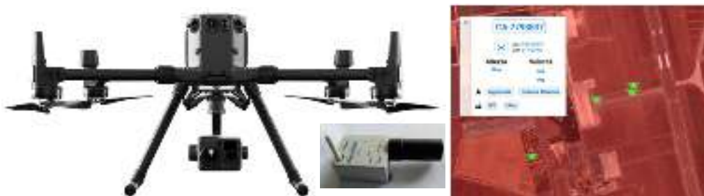
Figure 2-3: S1 - M300 RTK with Pollicino Pro Tracker and D-flight cartography with UASs / aircrafts tracking information with altitude reference (translated by ICARUS prototype service)
