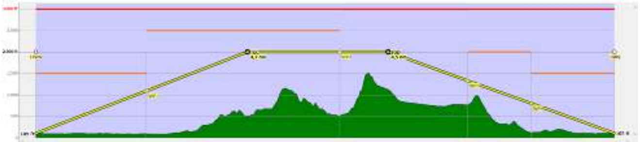
Figure 2-8: S1 - Elevation profile for C-172 aircraft Flight plan related to the training mission from RAINS club airfield (LIWS)
