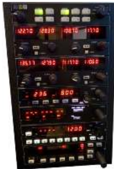
Figure 2-8 – Bendix King style avionics set integrated in Easy Flight main panel
