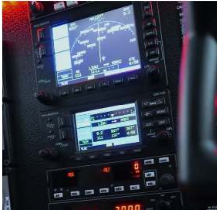
Figure 2-15 – GNS530 and GNS430 replica integrated in EasyFlight Cockpit main panel
